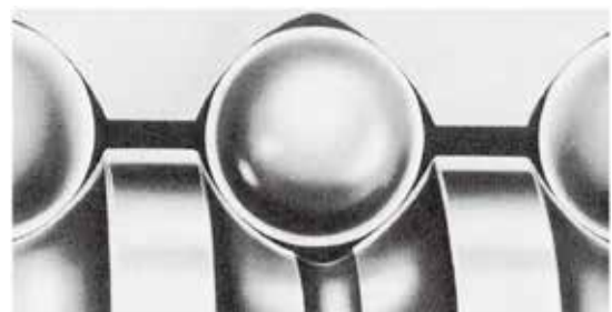
Ball screw groove profile
