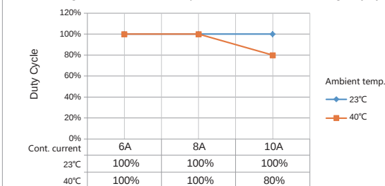
200W-Standard type Cont. running current , ambient temp. and recommended working duty cycle.
